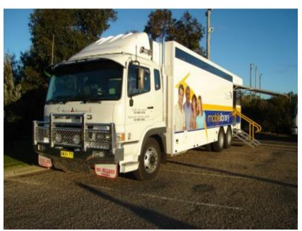
36. Australian mobile from Tafe at Dubbo in New South Wales This shows the rugged build and 'roo' bars for a vehicle that travels across the outback for up to 450 kms at a time
