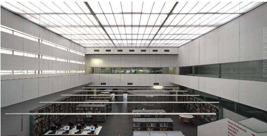
Alfons Soldevila has focused in the study and exploration of the capacities of the **translucent and transparent materials** in different projects. In the library of La Mina he starts from the idea of a translucent box which allows the entry of great quantity of light to the inside through the skylights on the roof and the slats all through the façades.
