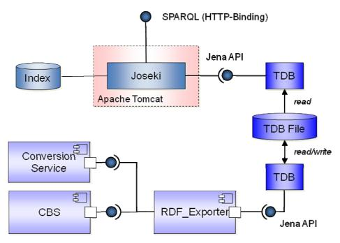
Figure 2: Current system architecture
