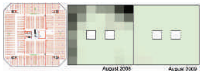
8. MGHI maps of 3 rd Floor Q1 for August 2008 and 2009. A comparison shows the reduced risk of mould in 2009. The darker colours correspond to higher MGHI.
