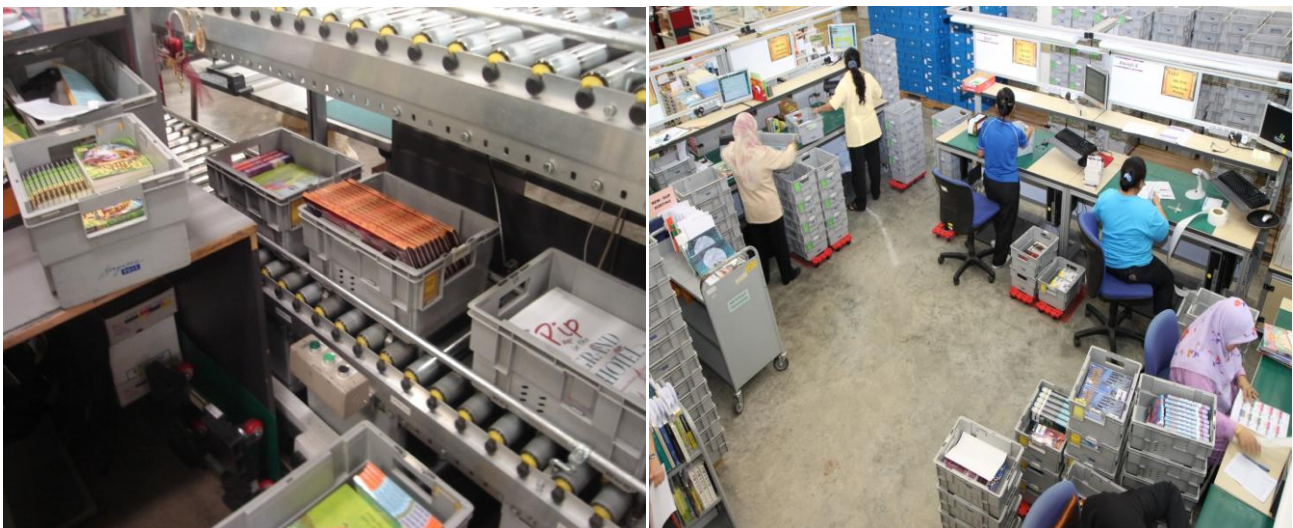
Figure 1: Previously, library materials were processed via a conveyor belt system (pictured left). With the new cellular manufacturing line (pictured right), multiple materials can be processed simultaneously, thus increasing productivity.
