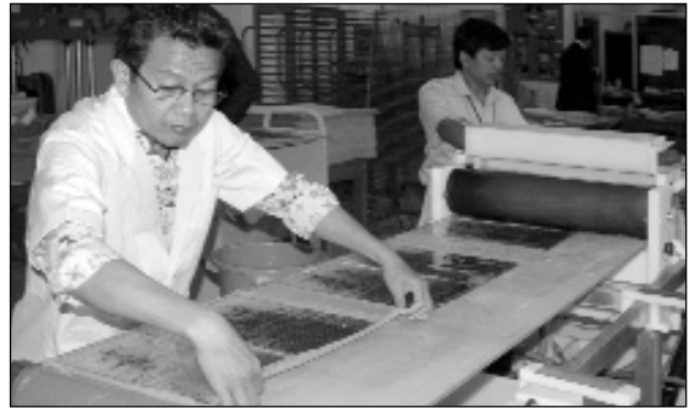
After disbinding, washing, and alkalizing with magnesium bicarbonate, Land Property record books are leaf cast to fill losses and add a 1 inch (2.5 cm) border to each sheet.
